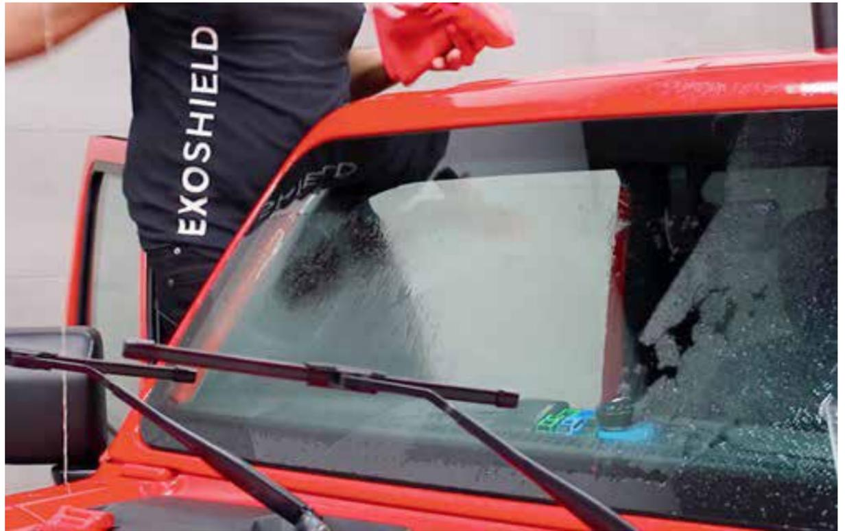
Alchemy's ExoShield windshield protection film being applied to an automotive vehicle.
