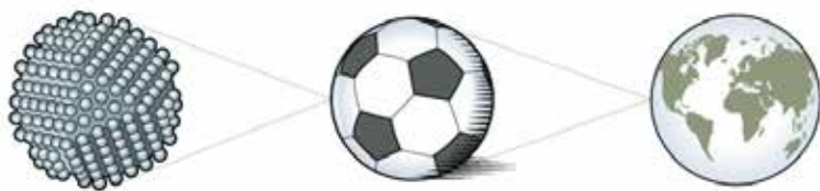
A quantum dot is a crystal that often consists of just a few thousand atoms. In terms of size, it has the same relationship to a football as a football has to the size of the Earth.
