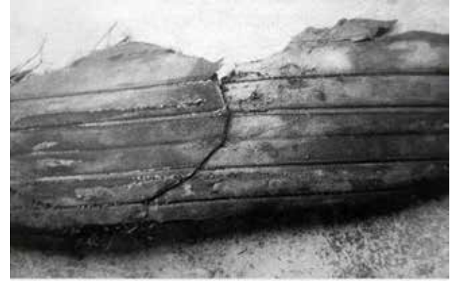
Found on runway 26R at Charles de Gaulle after the crash, this 4.5-kilogram (9.9-lb) fragment of Concorde's number 2 tire, punctured by debris left behind by another departing jet, had hurtled into the number 5 wing tank, causing an internal shock wave that ruptured the tank. (BEA REPORT, 60)
